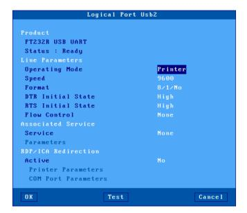
This USB logical port allows the adaptor to be configured: line parameters (baud rate, format...), service and RDP/ICA redirection. For more information see Chapter 3.5.1.
