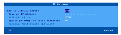
The option "Use TS Gateway Server" allows the name or the IP address of the RDS gateway server to be entered.
