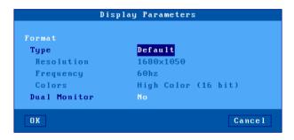
This box allows display settings (resolution, number of colors and frequency) to be set. The availability of these parameters depends of the **Type** value:
