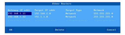
**Example 2**: router 1 is used to reach both networks (192.168.2.xxx and 192.1.1.xxx):
