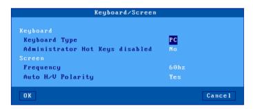
**Keyboard Type**: by default PC keyboards (102/105 keys) are supported by the AX3000, but other keyboards type are available for special use:
