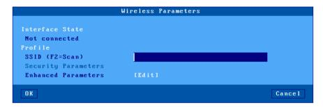
This box allows the wireless profile to be set-up (only one profile)
