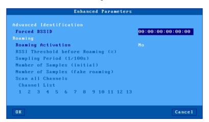
**Forced BSSID**: in event of multiple access points with the same SSID, this option allows a specific one to be selected via its MAC address (BSSID).
