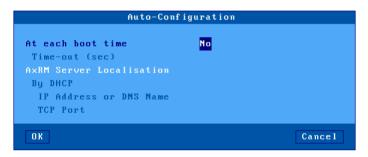
The 'time-out' parameter is the maximum number of seconds allowed for the terminal to load a new firmware/configuration. If nothing is received in this time the terminal boots up using existing current settings.
