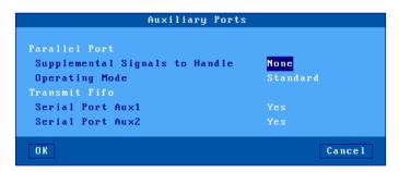
**Supplemental Signals to Handle**: the AX3000 checks the printer status by reading both the "Busy" and "Select-In" signals before printing. The AX3000 will not transmit data for printing if the printer handles only the "Busy" signal. This parameter determines whether the "Select-In" and/or "Paper Empty" signals will be selected in addition to the "Busy" signal (which is always used).
