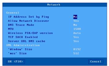
**IP Addr. Set by Ping**: this parameter allows or disables the AX3000 IP Address to be set by a ping command. (See Appendix A.8.6.)
