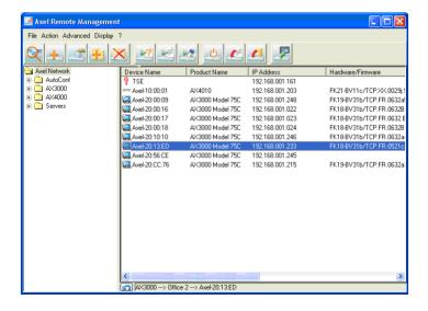
The AxRM software allows system administrators to manage and configure Axel TCP/IP products remotely over a network. The remote Axel device is selected by its IP address or network name. (The software can also assign an IP address to a newly installed terminal that has not had an IP address set)
