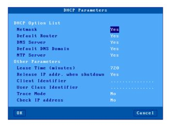
The "DHCP Option List" allows certain parameters to be automatically assigned by DHCP.
