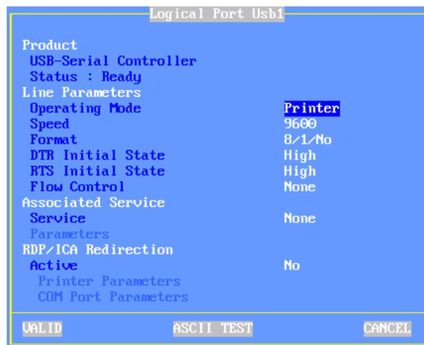
This USB logical port allows the adaptor to be configured: line parameters (baud rate, format...), service and RDP/ICA redirection. For more information see Chapter 3.5.1.
